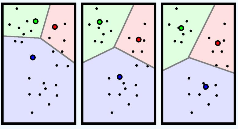
An example of the K-means algorithm separating data points into 3 clusters. Here, the clustering occurs in 3 iterations. Black circles represent data points, colored circles represent centroids, and points in the same colored region are in the same cluster.
